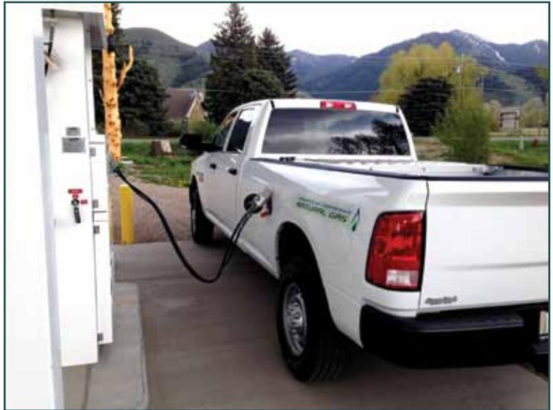
*TCD's new Dodge Ram 2500 bi-fuel pickup fueled by both natural gas and unleaded gasoline.*
